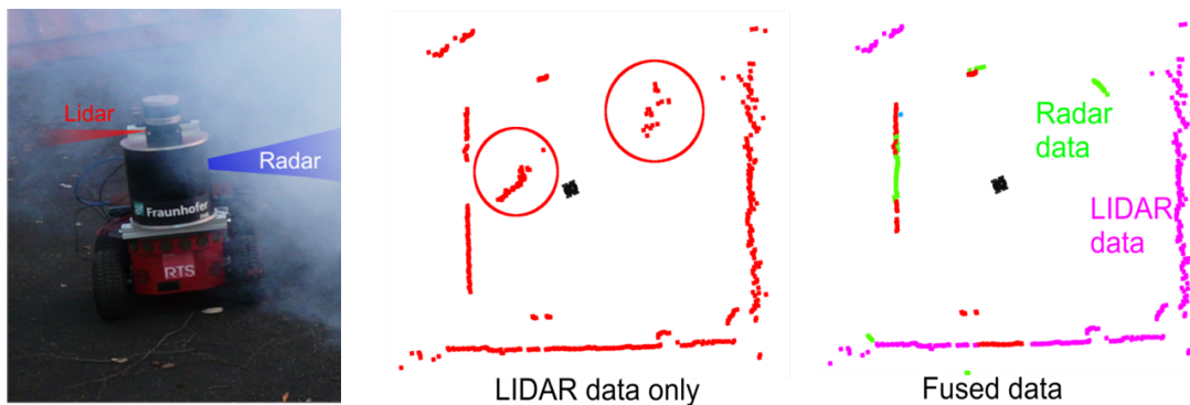
Figure 5: Data Fusion with Lidar and Radar; Integrated System (left), LIDAR data only (center), fused data (right)
