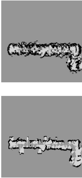
Figure 8: Above: This occupancy grid map is built from raw data of the lateration technique. The wide spread of the sensor data is caused by non point target situations. Below: This map is obtained from of the ASR technique.
