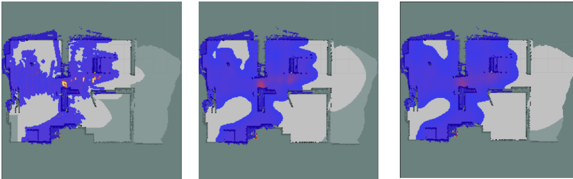
Fig. 16 Prediction of thermal information to three different time steps. The hot area in the middle of the map is a human.
