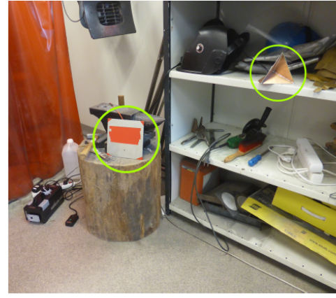
Fig. 6: Workshop environment with fog machine (left) and heat targets (marked with the green circles).
