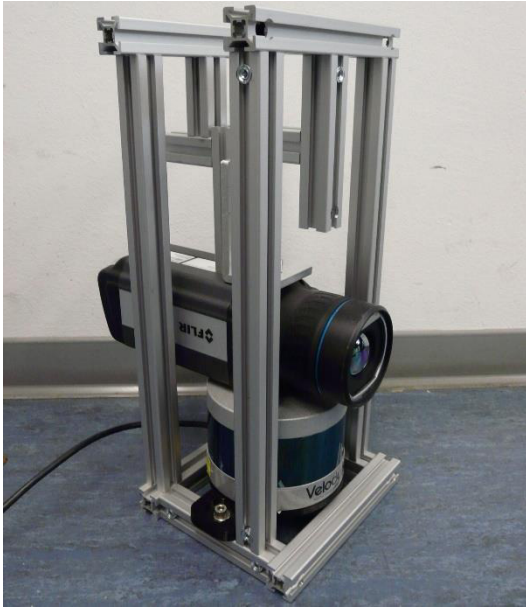
Figure 3: Rigidly mounted sensor stack consisting of thermal imaging camera (top) and 3D laser range finder (bottom).
