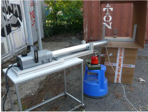
Figure 20: High-temperature smoke experiment: Smoke is carried through a pipe and heated by a gas burner. A cardboard frame serves as a windbreak. Inside the frame, there is a heated target.
