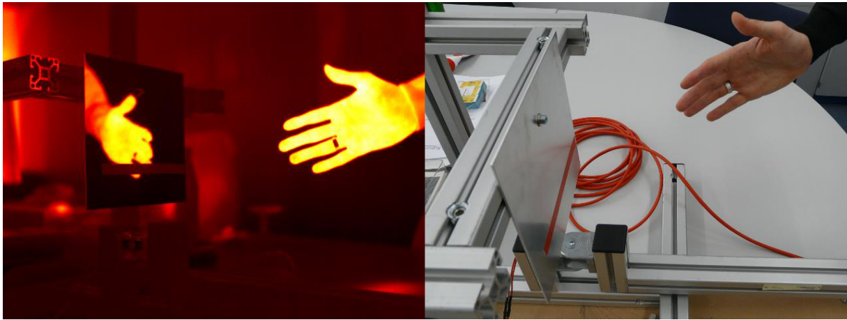
Figure 2: Exemplary thermal reflection of a human hand on a polished aluminum plate (left). For comprehension, the scene is also shown as a RGB image (right).
