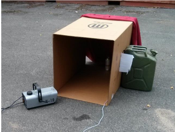
Figure 17: Low-temperature smoke experiment: Smoke is carried into a cardboard frame that serves as a windbreak. Inside the frame, there is a heated target.
