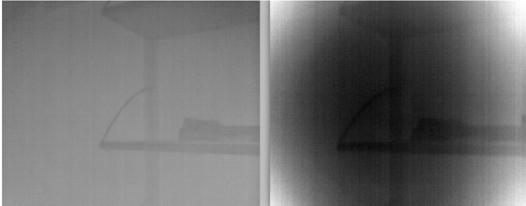
Figure 3: (left) A sample of the thermal image taken by the intact camera. (right) The corresponding thermal image taken by the damaged camera. A radial darkness can be observed on the image which is due to a malfunction of the camera.
