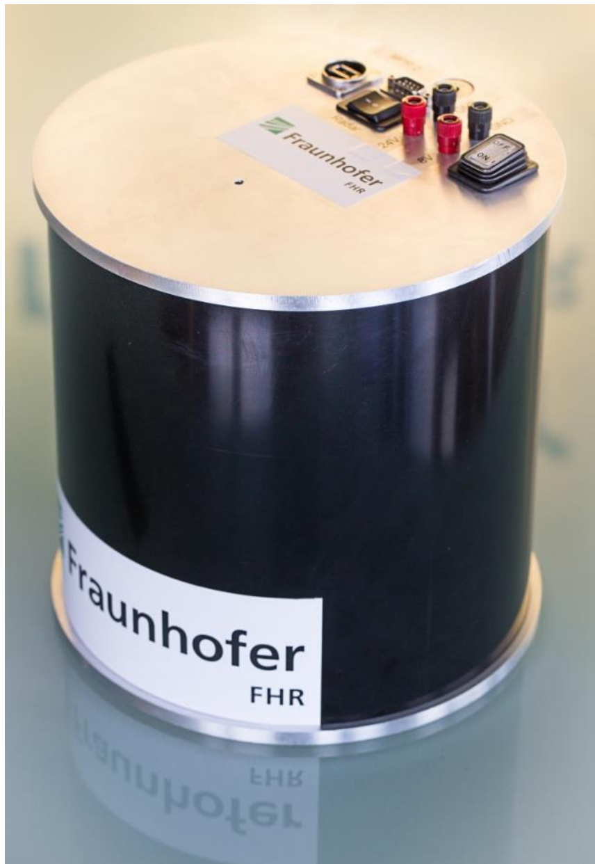
Fig. 3.12: Photograph of 2D MPR with mounted radome
