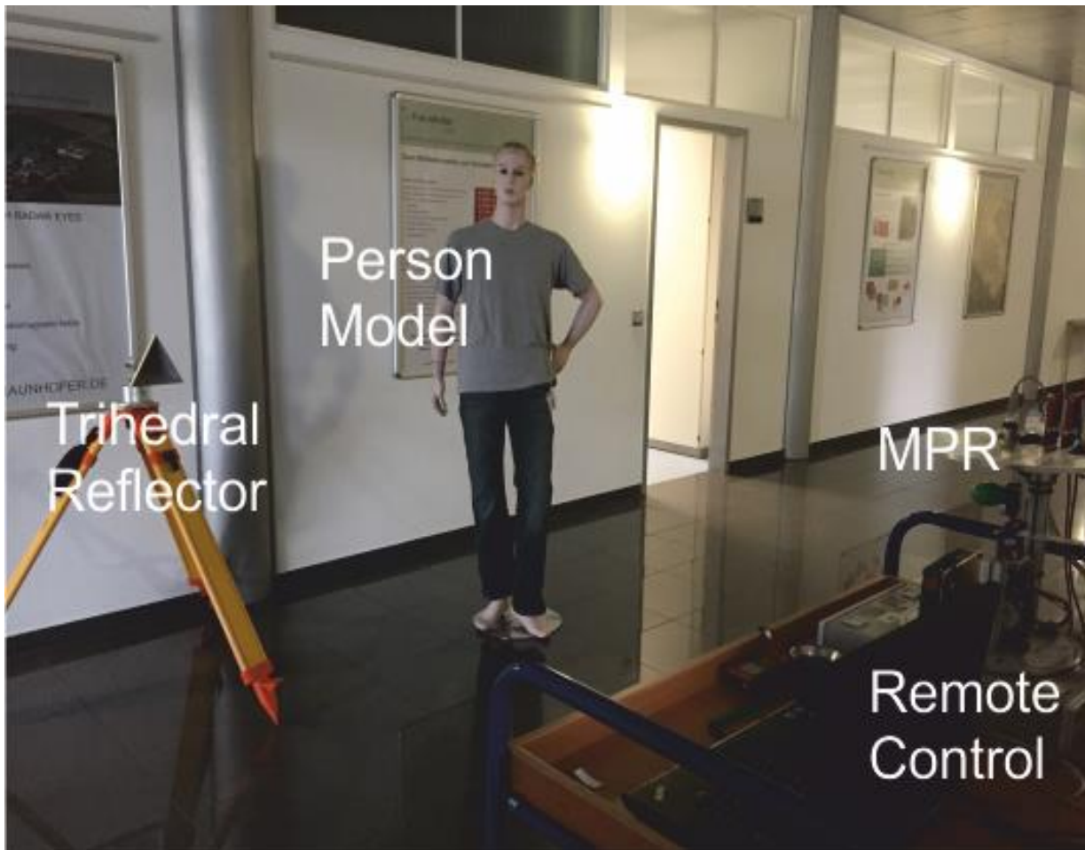
Fig. 3.19: Measurement scene for experimental MPR characterization
