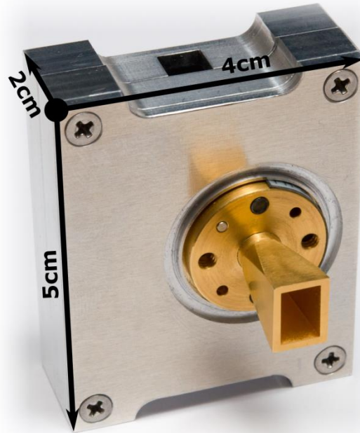
Fig. 2.5: Photograph of Radar Module in Case
