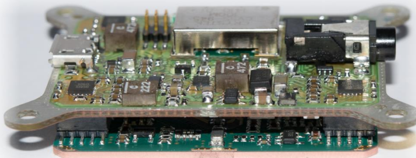
Fig. 2.6: Photograph of frontend and backend of the radar module
