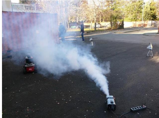
Fig. 16 Robotic Platform with MPR and Velodyne VLP-16 in a smoke scenario.
