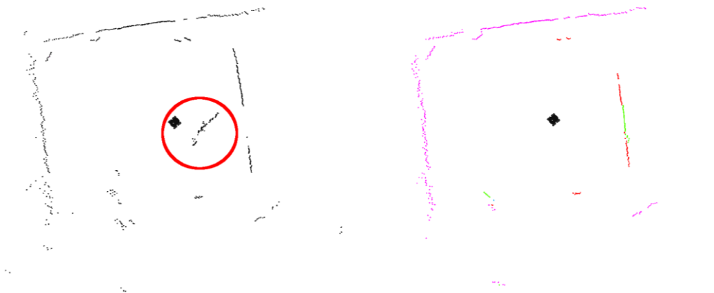
Fig. 17: Left: The robot and detected smoke is visible (inside the red circle): The LiDAR reports smoke in the same way as an obstacle. Right: The fusion algorithm combines Velodyne VLP16 and MPR measurements and replaces LiDAR points that are affected by smoke with radar points (green), which combines the advantage of both sensors – the higher accuracy of the LiDAR and radar measurements that are not disturbed by smoke.
