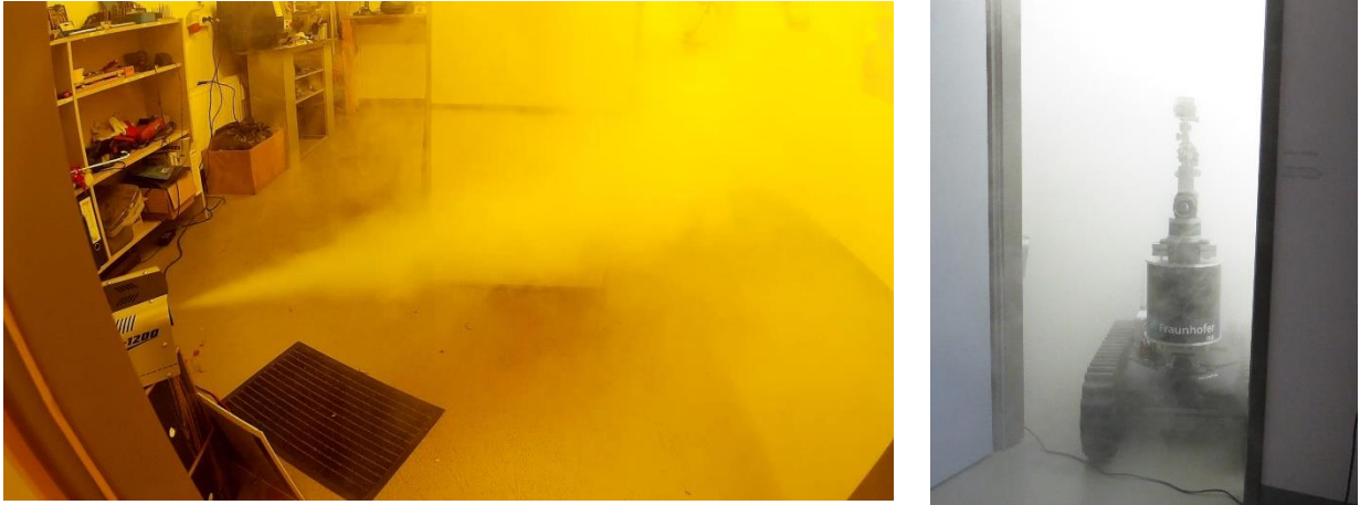
Fig. 21 In order to test the sensor fusion's capability to handle the Type II effect, we filled a room with very dense fog.
